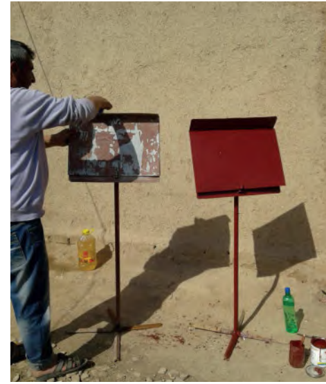
Repair work of one of the reading stands: welding the metal structure and repainting
